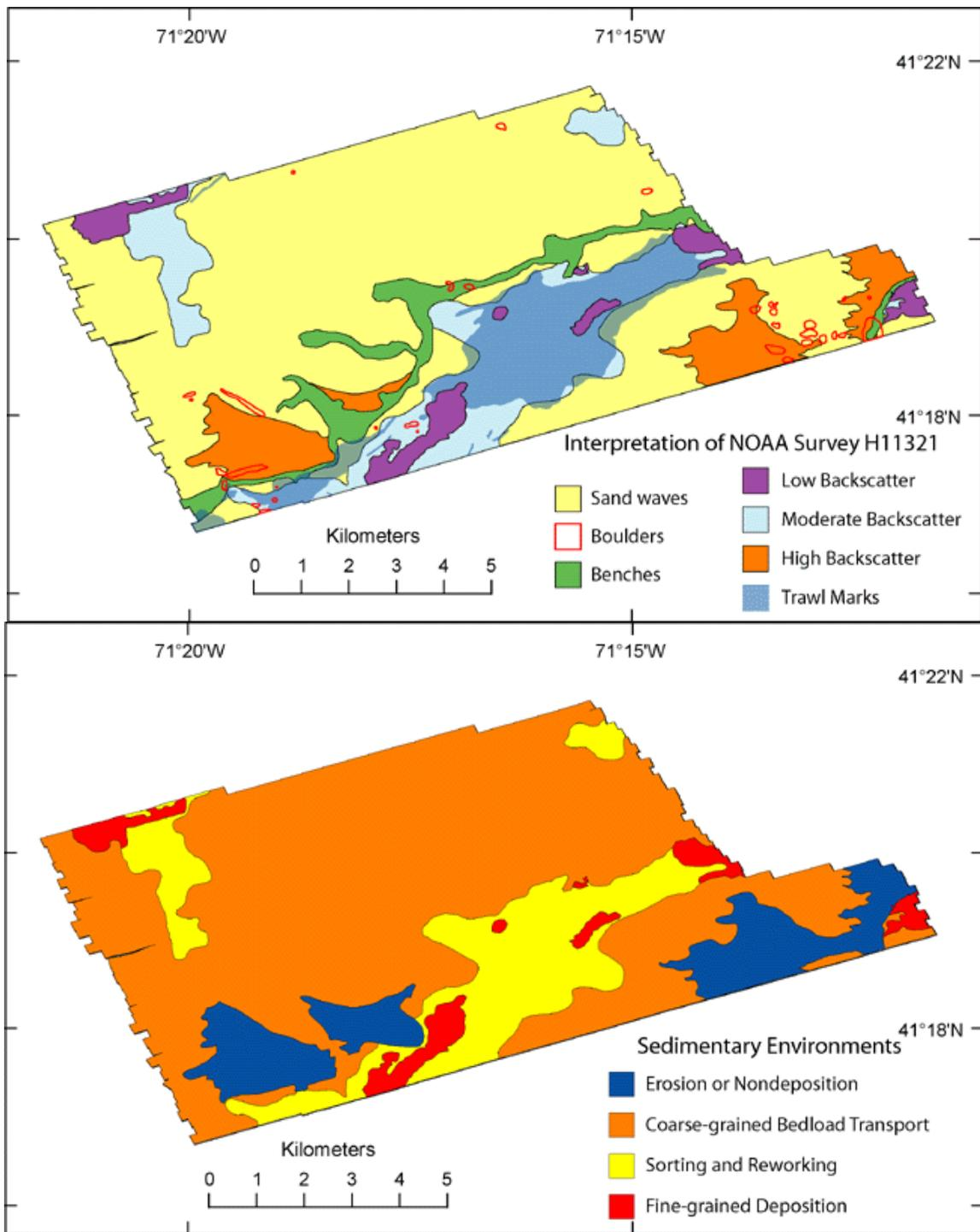
**Figure 2.4.** Bottom characteristics in a section of Rhode Island Sound as interpreted from sidescan sonar images (McMullen et al. 2008; their Figure 14 (upper) and Figure 10 (lower)). Note the large expanses of sandy area punctuated by scattered boulders in the upper panel. Yellow area in the lower panel shows more stable habitat areas, with orange (sand areas in the upper panel) areas being more transitory.
